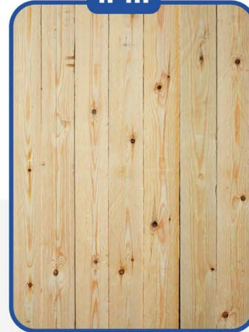
Boards feature robust and secure knots, with four sharp-edged faces, free of splits.
